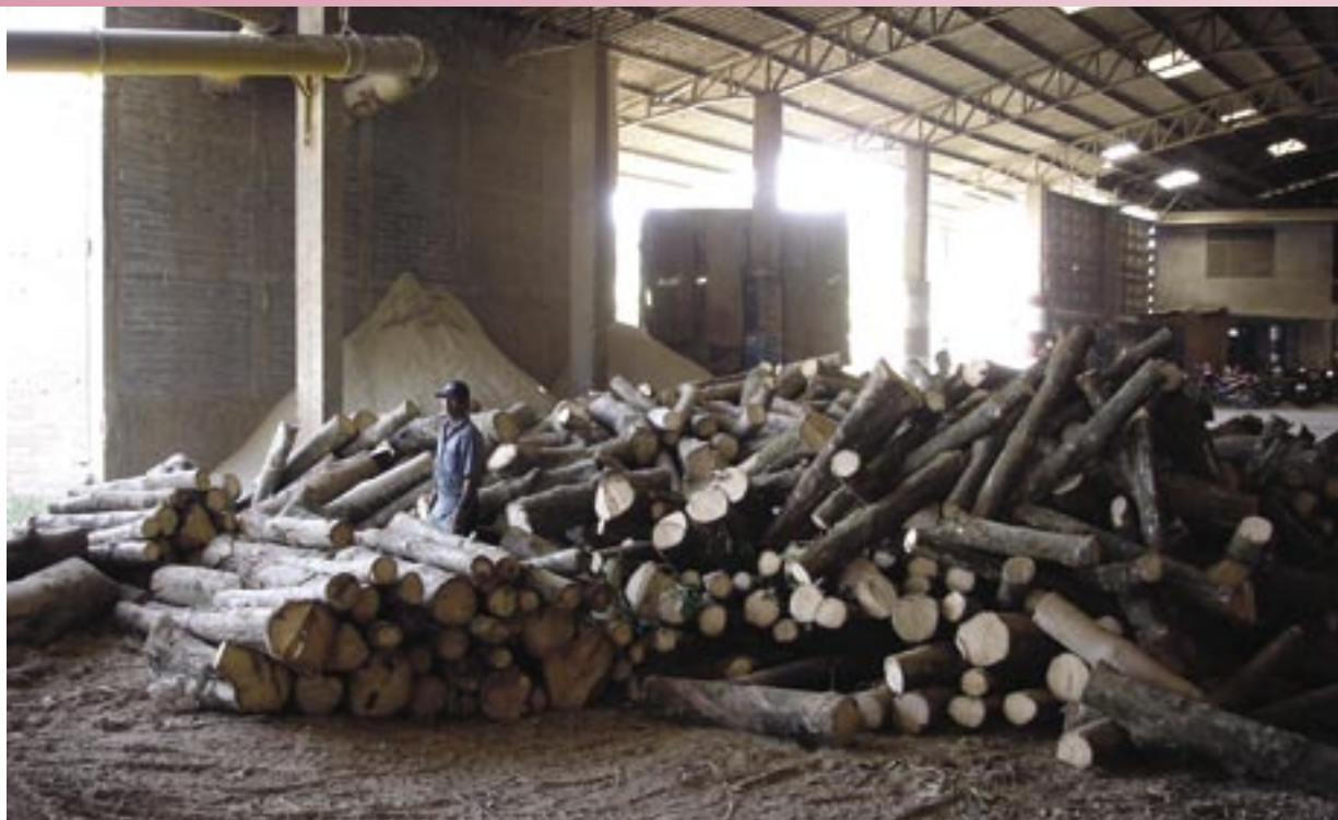
Log jumble: the mission found that log yards are not organized to make best value of the raw material. Photo: M. Simula
